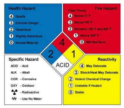
Figure 2.4- NFPA Hazard Rating System
